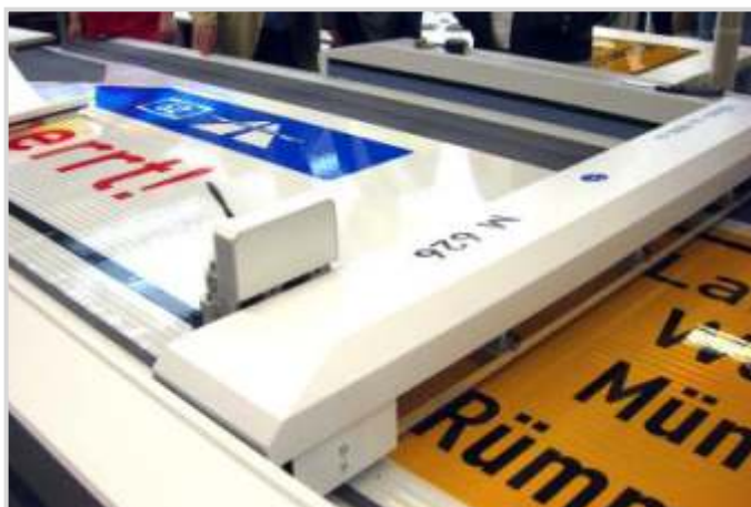
Manufacturing of a traffic sign on a special printing machine
